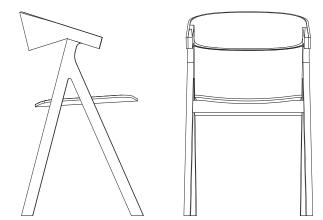
OVERALL HEIGHT 780 SEAT HEIGHT 460 OVERALL WIDTH 500 OVERALL DEPTH 520
